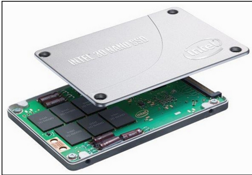
An exploded view of an SSD. Image courtesy: Intel Corporation
