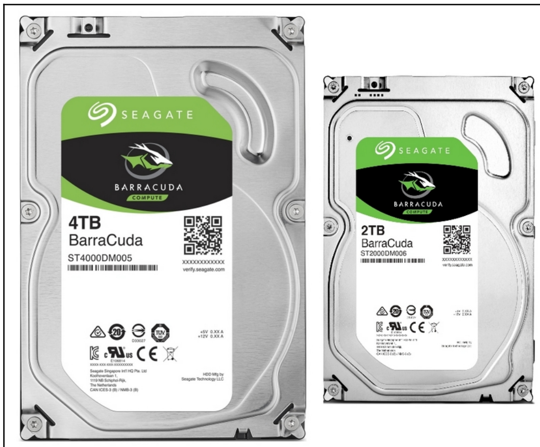
A comparison of a 3.5-inch LFF (left) and a 2.5-inch SFF (right) Image courtesy: Seagate Technology, LLC
