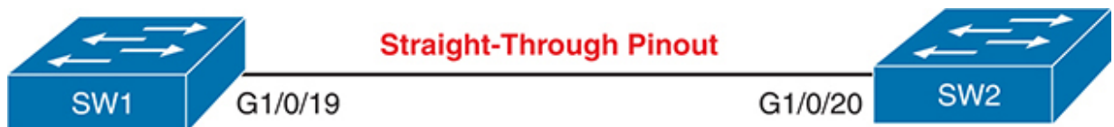
Figure 7-6 Switch-Switch Link That Needs Crossover but Uses Straight-Through Cable
