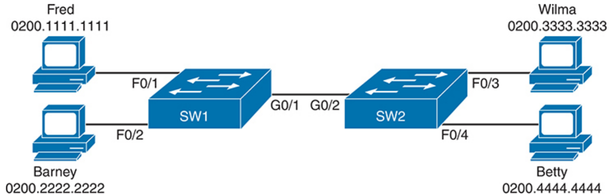
Figure 5-10 Two-Switch Topology Example
