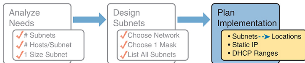
Figure 11-19 Facts Supplied to the Plan Implementation Step
