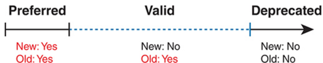
Figure 28-10 SLAAC Preferred and Valid Lifetimes for One Temporary Address
