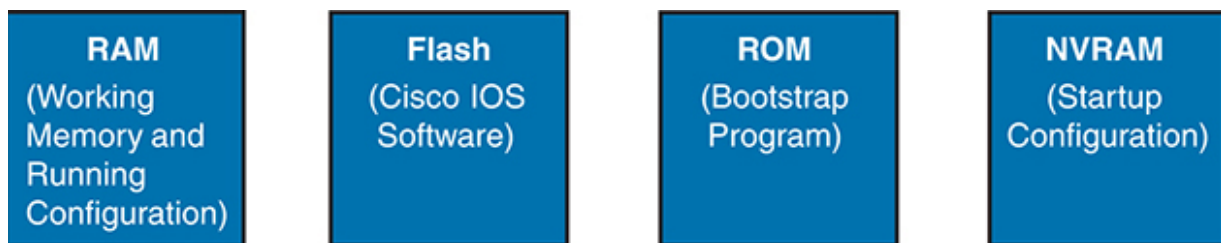
Figure 4-13 Cisco Switch Memory Types
