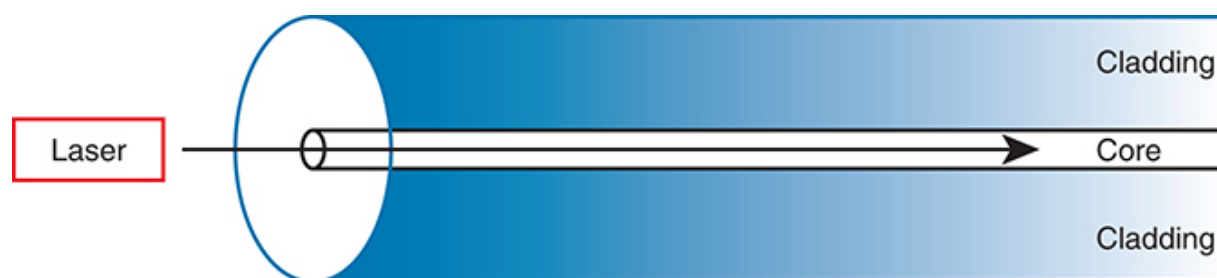
Figure 2-16 Transmission on Single-Mode Fiber with Laser Transmitter
