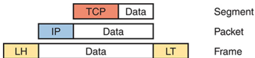
Figure 1-13 Perspectives on Encapsulation and “Data” *
