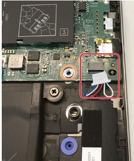
FIGURE 9.5 Disconnecting the speaker cable
