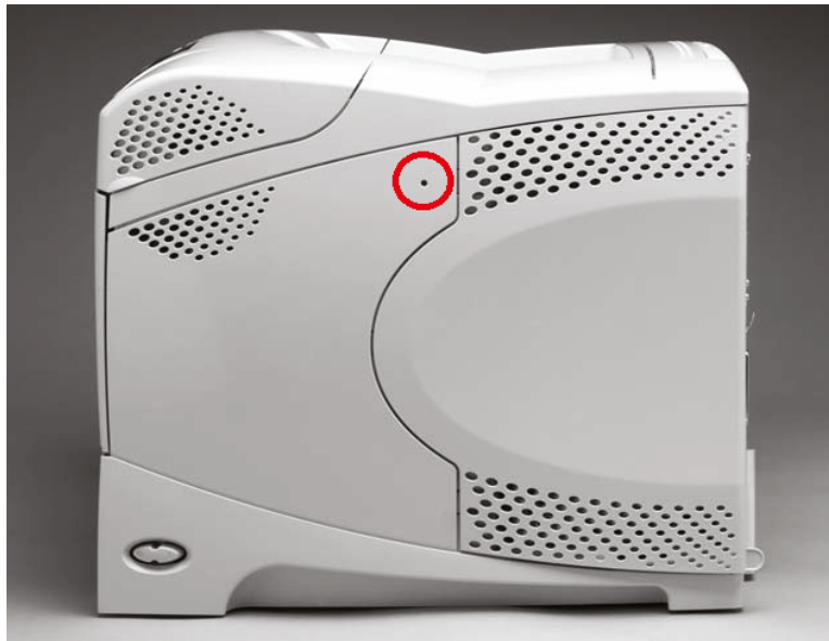
FIGURE 12.18 Print engine self-test button location. The location will vary on different printers.
