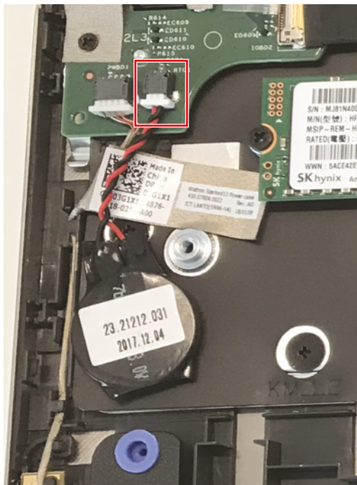
FIGURE 9.39 Disconnect the CMOS battery.
