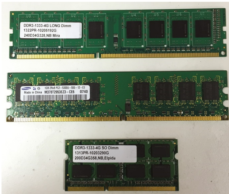
FIGURE 1.35 DDR3 SODIMM vs. DDR3 and DDR2 DIMMs
