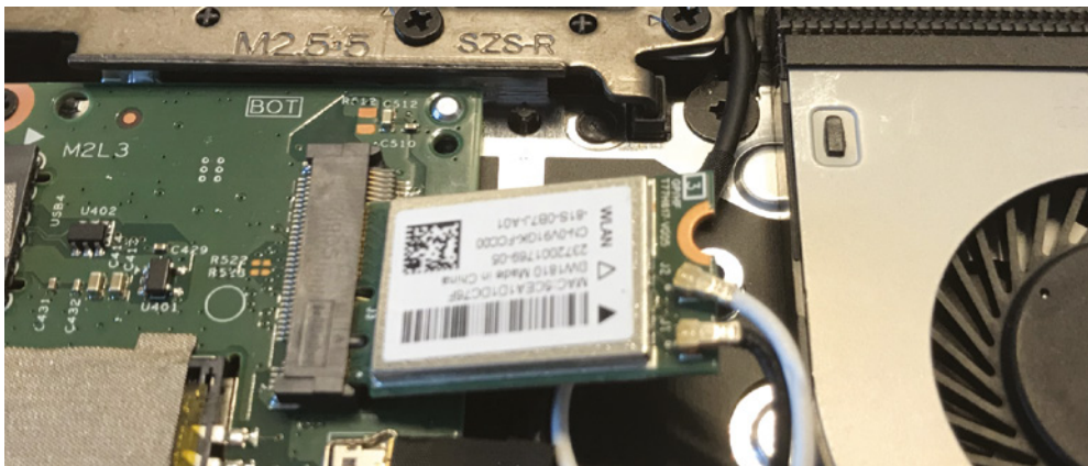
FIGURE 9.38 Disconnect the two antenna wires.
