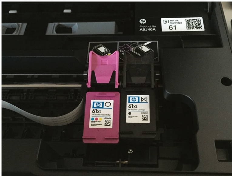
FIGURE 4.3 A print head carriage (holding two ink cartridges) in an inkjet printer
