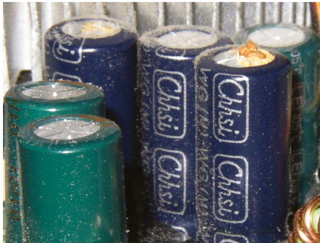
FIGURE 11.3 Distended capacitors on a motherboard
