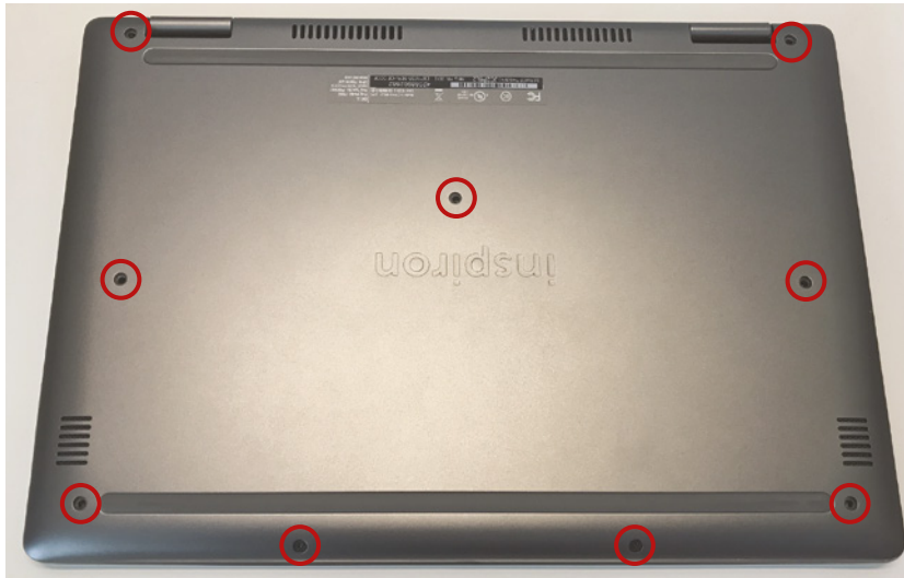
FIGURE 9.3 Removing nine screws to take off the bottom cover
