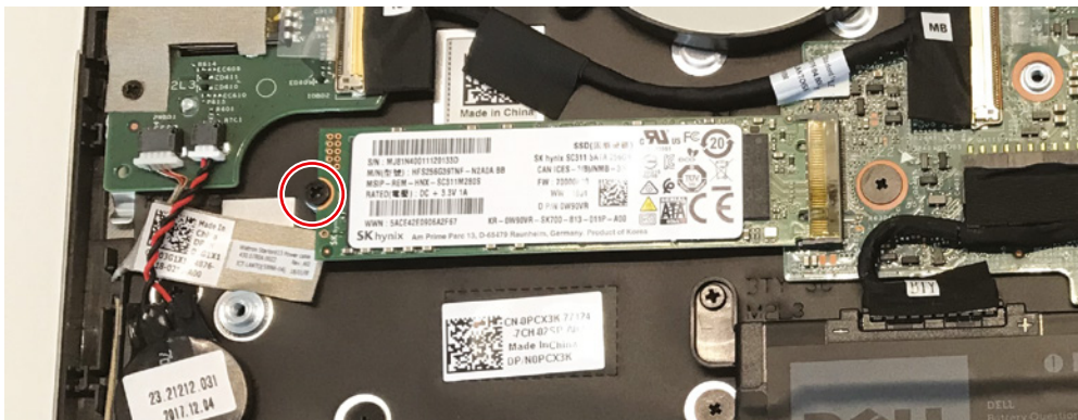
FIGURE 9.22 Removing an M.2 SSD
