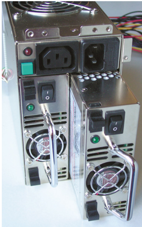
FIGURE 2.36 Hot-swappable redundant PSUs
