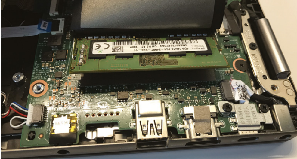
FIGURE 9.17 Removing a SODIMM
