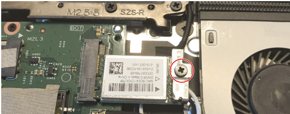
FIGURE 9.37 Removing the wireless NIC
